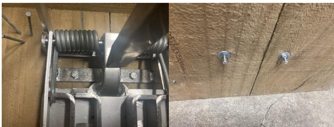
Figure 2. For test 2 the modified trap was bolted into the tunnel base (left) with a washer and nut assembly, securing the bolts on the underside (right). A setting tool was used to set the trap.
