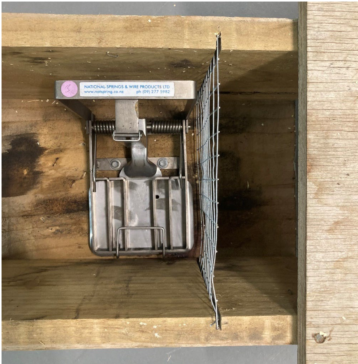
Figure 1. Unset BT200 kill trap in a Haines Pallets single-entrance tunnel. The lid has been unscrewed and opened to view the trap from above. The trap was firmly screwed to the tunnel base. Standard rodent feed pellets smeared with either Nutella® or smooth peanut butter were placed to the left of the trap.
